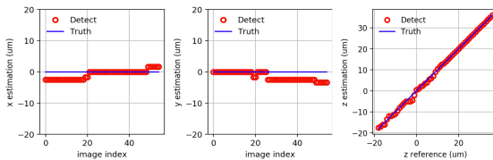
(c) Localization performance of the proposed CISTA-net. RMSE for x, y, z position detection is 1.60, 1.98, 0.82 \mu\text{m} , respectively.
