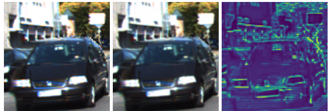
Fig. 6: Detail from views to illustrate the contribution of the Refiner. From left to right: prediction from DBP, final prediction, confidence map.
