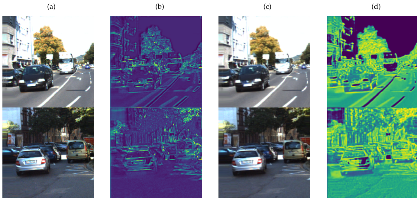
Fig. 8: Elements of comparison for constraint set on the confidence map (yellow in confidence maps means low-confidence in DBP prediction). a) Prediction when FB-constraint is set. b) Corresponding confidence map. c) Prediction when no FB-constraint is set. d) Corresponding confidence map.
